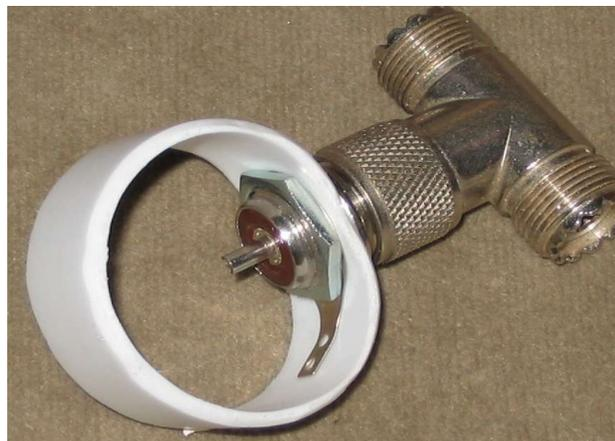
The SO239 fitted. The "T" piece is used to hold the SO239 while the nut is tightened.
