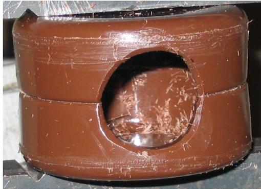
Clamp the two gliders into a vice and mark out the hole for the coax connection. This hole has to be big enough for the screw on part of a PL259 to go through with a bit of clearance.
