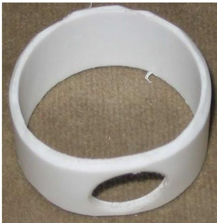
The PVC pipe with the hole cut for the SO239. Notice the chamfer on the "ends" of the pipe.
