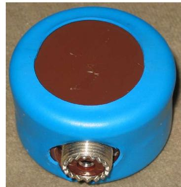
Check that everything fits as it should, apply PVC weld glue to the mating surfaces of the two gliders, and to the inside of the gliders and the outside of the PVC pipe where the two will touch, clamp it in the vice for a few hours, and finally cover the completed transformer with a protective piece of heat shrink tube.
