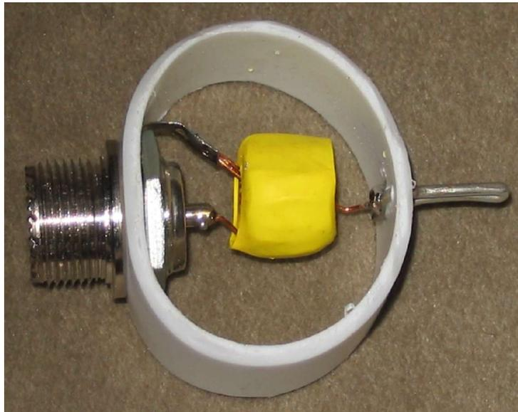
The transformer has had heat shrink tubing put over it, and has been mounted to the wire terminal and the SO239.
