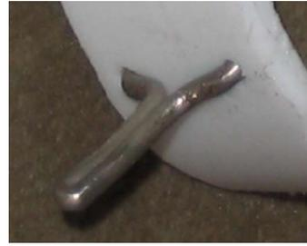
On the opposite side of the pipe to the SO239, two holes are drilled and a terminal fashioned for the wire antenna out of some 16SWG copper wire. The reason the SO239 and the terminal are used instead of going straight into the transformer is to enable the coax to be disconnected and used for another antenna to save the amount of coax carried, and to secure the wire and coax against twisting.
