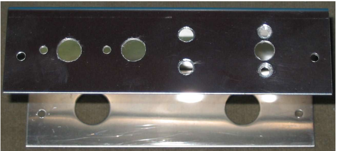
The initial drilling. Between the two large holes on the back for the SO329s I added a phono socket for a wire antenna connection.
